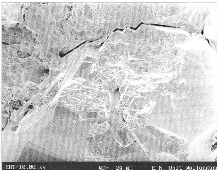
SEM micrograph showing intense 'transport controlled' etching within the early Permian Snapper Point Formation at Jervis Bay, south of Sydney, Australia. Much of the overgrowth is highly corroded, though other areas are only slightly etched. Field of view 250µm.
